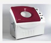
Salt fog is a specialized test used to evaluate the resistance to corrosion of paints, coatings, and metal structures as well as effects on electrical systems. Our chamber provides exposure to a salt intensive atmosphere at temperatures matching the proper specification. Other corrosive elements may be used for further corrosion testing.
